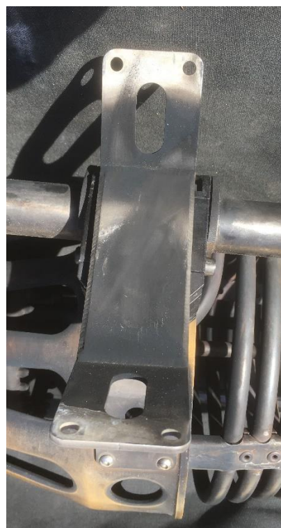
Fig 2. Hanger with doubler plate.
